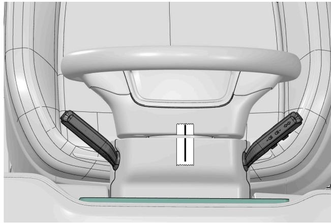
5. With vehicle in the “ON” position, perform steering wheel lash inspection
