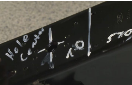
Figure 3 Repairer Anton Verwijst utilized the center of the cradle-bolt hole as a fixed reference point to obtain an additional measurement moving toward the back of the vehicle.
