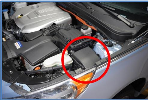
3. Remove the IG1 relay (tan). Refer to the illustration for relay location.
