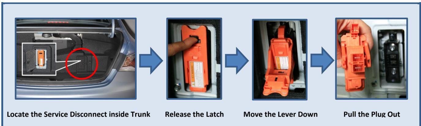
**Secondary Method:** Remove fuse or relay, disconnect the 12V Auxiliary Battery, and remove the Service Disconnect Plug.
